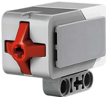
When the button is pressed on the touch sensor, an electrical signal is sent to the microprocessor. This signal can then be used by the program to follow a specific set of instructions. For example, use the program in Fig 2 below to instruct the robot to move forward until the touch sensor is pressed, stop and move backwards 3 rotations.
